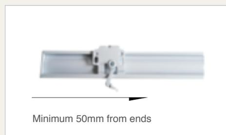
Plan where you will position the brackets on the blind rail. A bracket should be positioned at either end of the rail but at least 50mm in from the end. Position any other brackets along the rail spaced as equally as possible. When you have decided where each of your brackets will be located measure the position of each of the brackets along the blind track.
