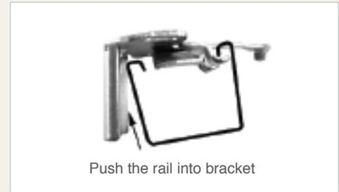
Offer up the blind rail to the brackets. Hook the lip on front edge of the rail over the protruding lips on the brackets.
