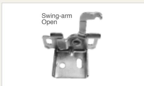
The brackets have a '**swing-arm**' mechanism. Before using the brackets make sure the swing-arm moves freely. Move the swing-arm into the 'open' position.
